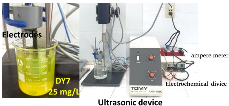
100 101 Figure 1A. ultrasonic, electrochemical, and sono-electrochemical experiments setup.
