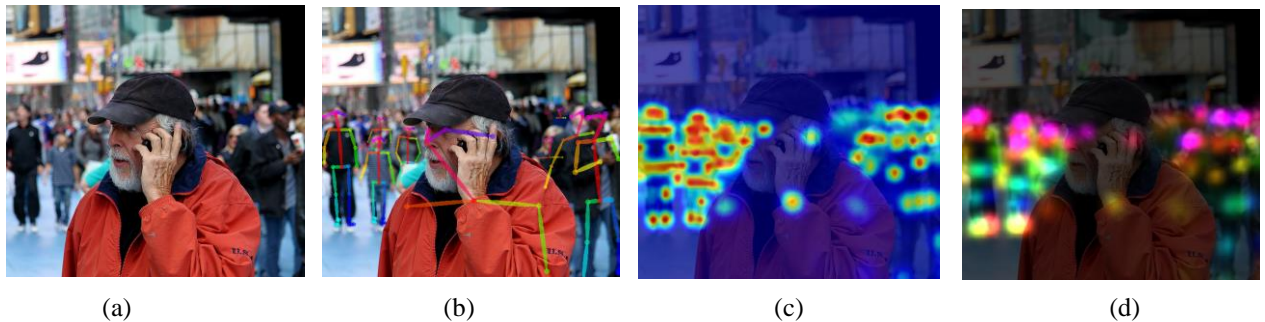
Fig 2. Extract (b) skeleton data, (c) Part Confidence Maps and (d) Part Affinity Fields from an (a) image
