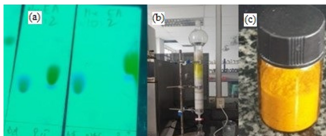
Figure 3. (a) TLC of coumarin ( 3 ) (left side) and bromo reaction (right side) in EA:He = v:v = 2:10; (b) chromatography of impure coumarin ( 4 ); (c) pure solid of coumarin ( 4 )
