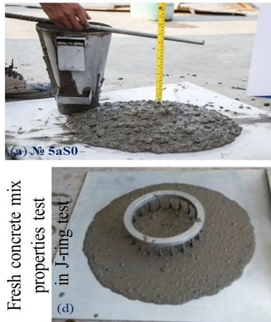
Figure 4. Tests for the workability of concrete mixtures: (a) Slump cone test or spreading (slump flow) test for concrete; (d) Limited spread measurement test.
