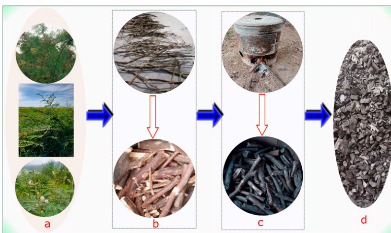
FIG. 1. Biochar production process: (a) Mimosa trees, an invasive species, used as the raw material; (b) shell and leaf removal, followed by drying and cutting into 7–8 cm pieces; (c) furnace operation and biochar formation after 2 h of pyrolysis; and (d) final biochar product with a particle size of ~1–5 mm.
