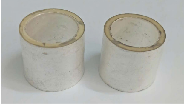
Fig. 15. The image of the cylindrical transducer after electrode coating.
