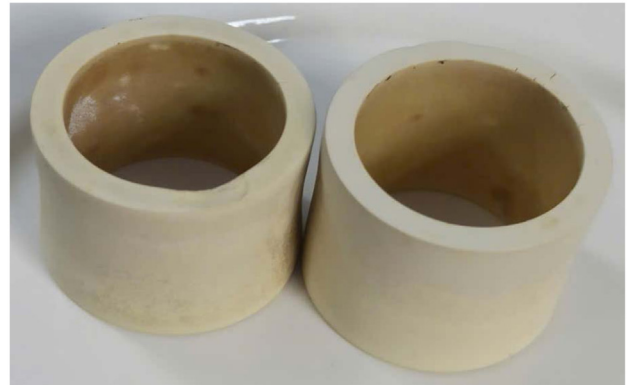
Fig. 14. Cylindrical - shaped transducer after sintering at 1150 °C for 3 hours.
