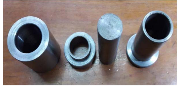
Fig. 13. Image of the cylindrical pressing mold.
