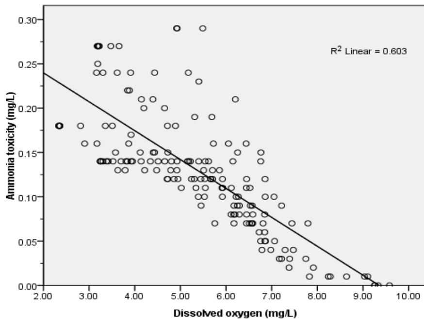
**Fig. 5.** Correlation of NH<sub>3</sub> toxicity removal and DO enhancement in all treatment by five mechanical methods
