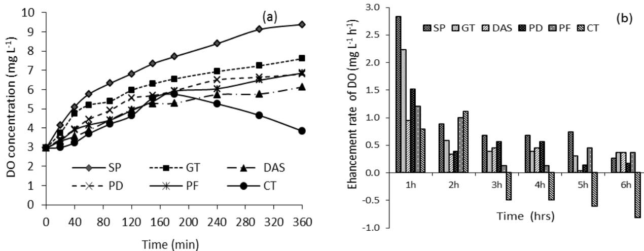
**Fig. 2.** (a) DO enhancement during 6 hours treatment and (b) rate of DO change per every hour in five treatment methods and control (SP: Splash board; GT: Gutter; DAS: Diffuse aerator system; PD: Paddlewheel; PF: Porcupine-fan; CT: Control).
