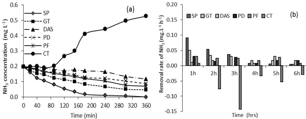
**Fig. 4.** (a)NH<sub>3</sub> removal during 6 hours treatment and (b) the rate of NH<sub>3</sub> change in every hour in five treatment methods and control (SP: Splash board; GT: Gutter; DAS: Diffuse aerator system; PD: Paddlewheel; PF: Porcupine-fan; CT: Control).
