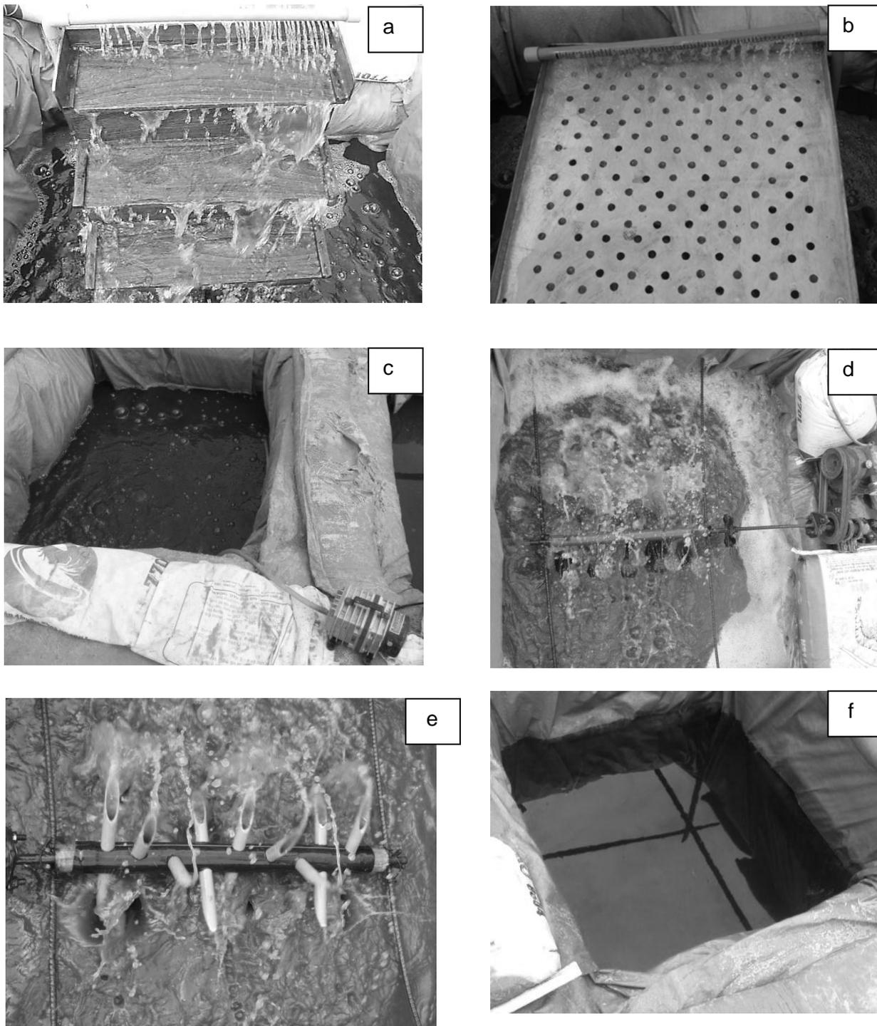
**Fig. 1.** Five mechanical equipment's design and a control used in the experiment (a. Splash board; b. Gutter; c. Diffuser aerator system; d. Paddlewheel; e. Porcupine-fan; f. Control).
