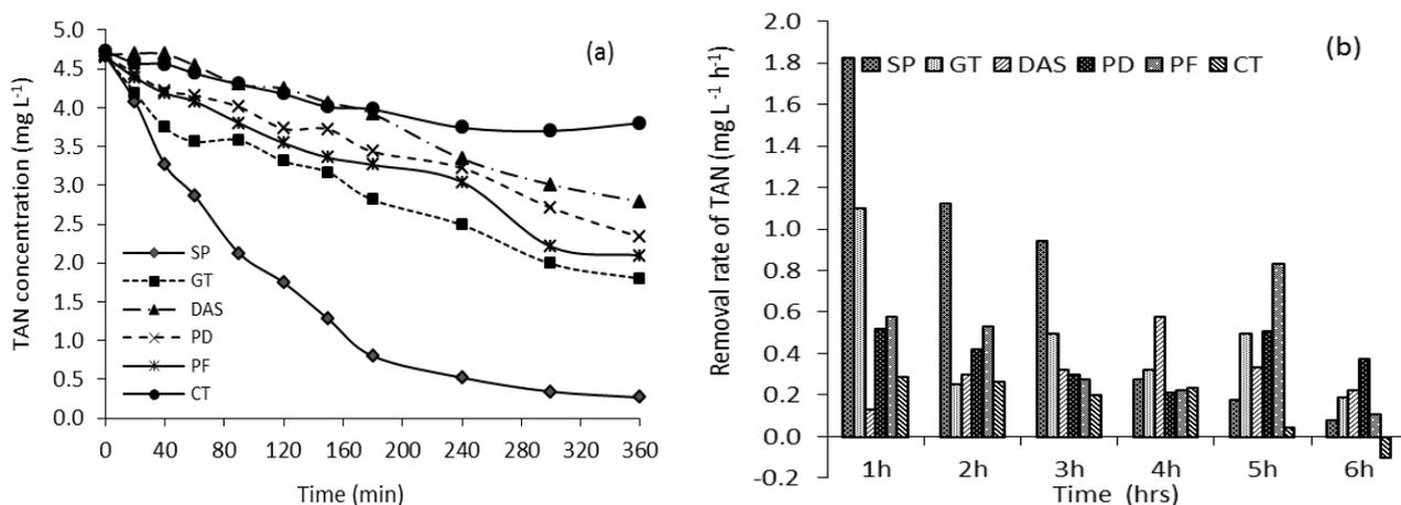
**Fig. 3.** (a) TAN removal during 6 hours treatment and (b) rate of TAN change in every hour in five treatment methods and control (SP: Splash board; GT: Gutter; DAS: Diffuse aerator system; PD: Paddlewheel; PF: Porcupine-fan; CT: Control).
