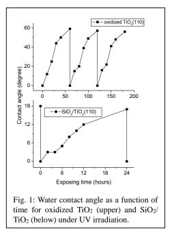
The almost fully-covered  $SiO_2/TiO_2$  surface showed the change from 0° to 16° after 24 h in dark. Note that the irradiation changed the wettability of not only oxidized TiO<sub>2</sub> but also  $SiO_2/TiO_2$ . The photo-induced holeelectron pairs in TiO<sub>2</sub> and their tunneling can contribute to the super-hydrophilicity. We will discuss them in detail.
